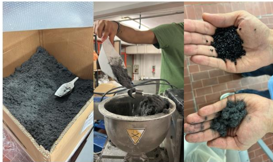
Safety belts powder from grinding
