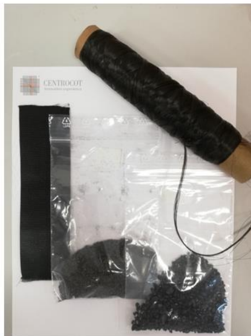
Safety belts → Powder → Pellets → Yarn
